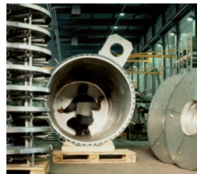
Installation of a slit tray
