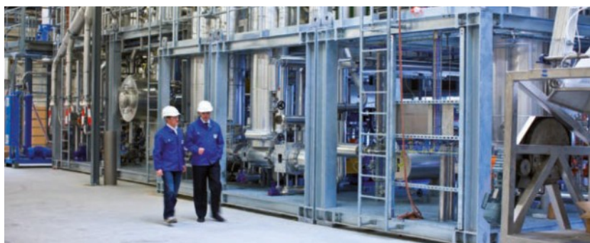
Skid mounted production unit for biodegradable polymer (PLA)
